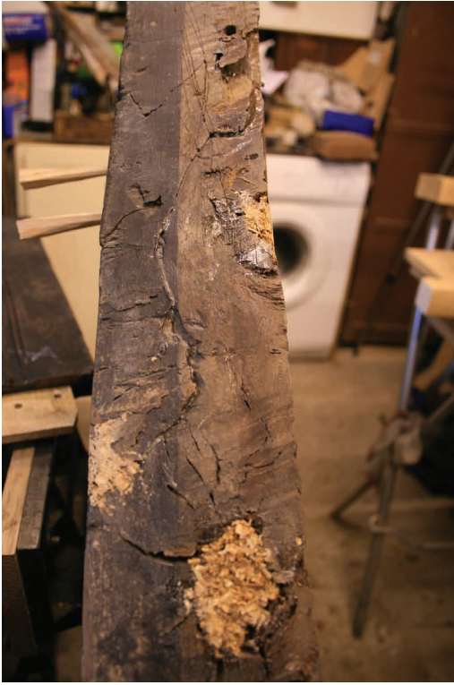
12 The back right stile, showing the very poor quality of timber used. The author
