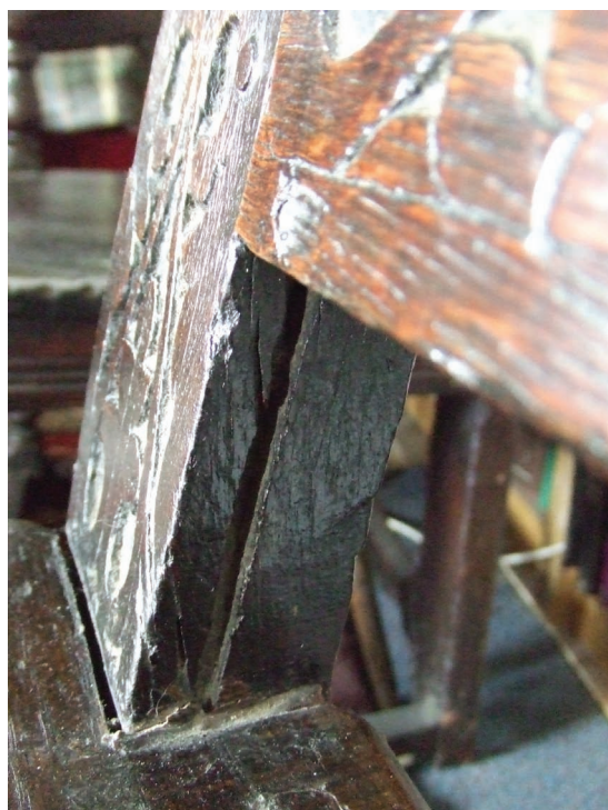
11 Detail of chair 3D, showing the groove in the left rear post made by the joiner's plough plane. Note how the groove gets shallower as the plane works back. John Gall
