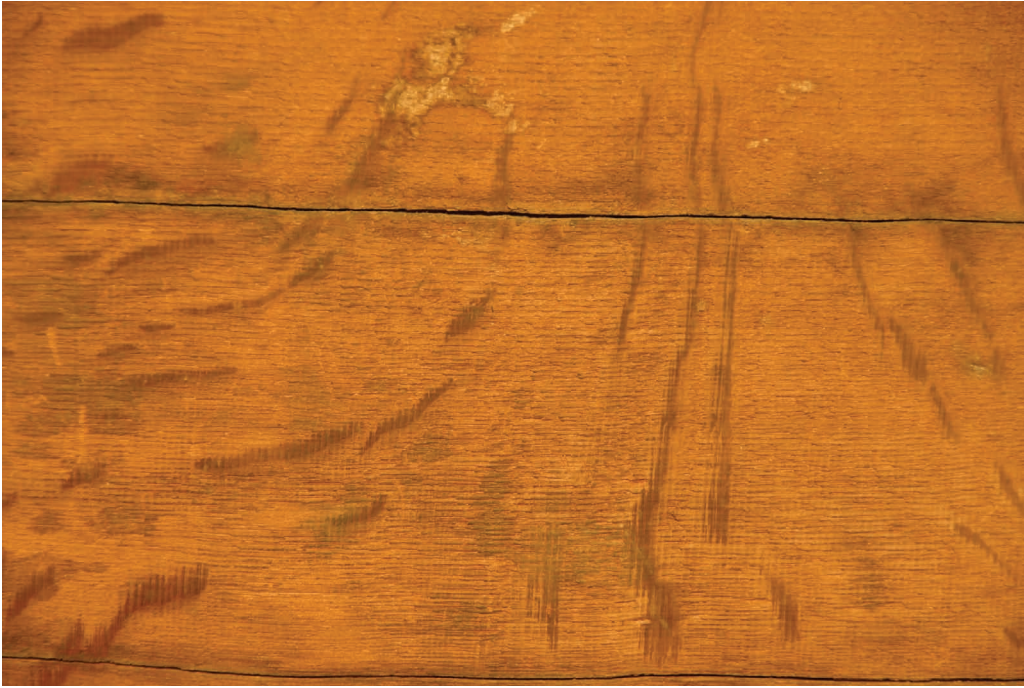
3 Underside of the seat of the Haughton-le-Skerne chair, showing the characteristic, closely spaced parallel kerfs of a Dutch multi-bladed wainscot saw. Adam Bowett
