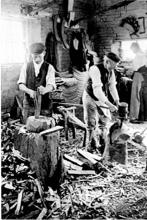
5. 'Butts' being split into 'billets' using a 'beetle and wedge'. In a Wycombe workshop, 1922
