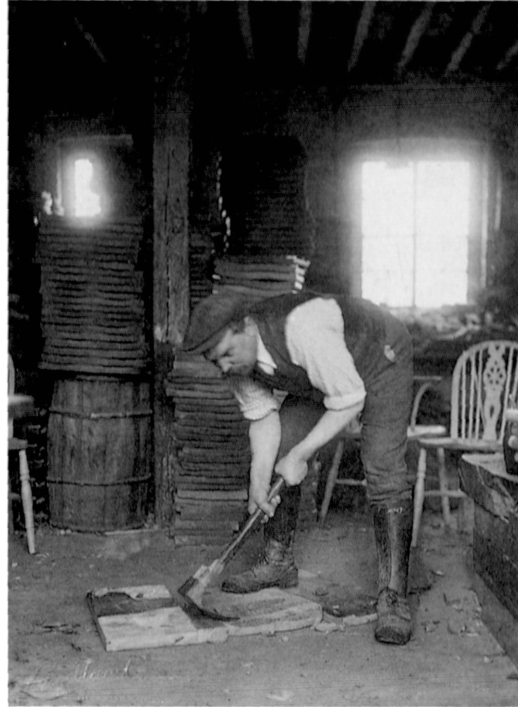
6. Adzing the seat with a chairmaker's adze, known locally as 'bottoming'
