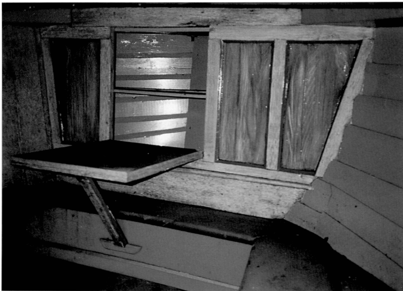
13. Leeds and Liverpool long boat Scorpio , aft. Table, locker and reversed clinker lining Boat Museum, Ellesmere Port
