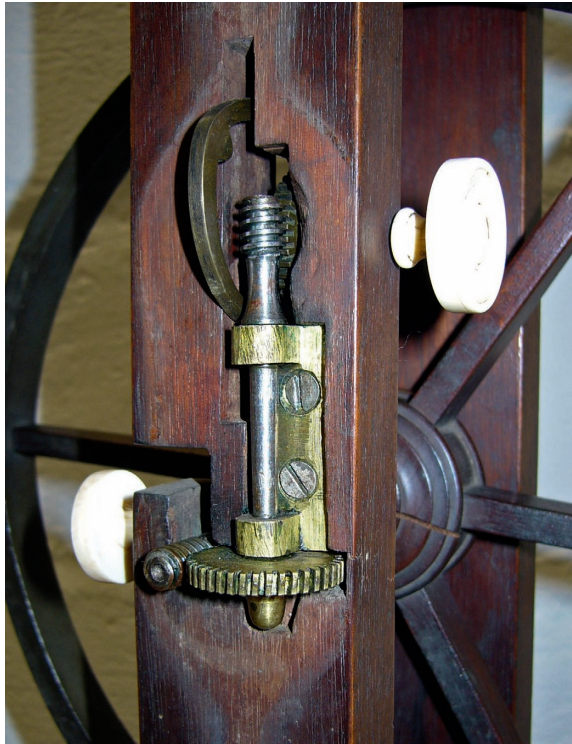
26 Detail of Figure 24, showing the Antis Mark 3 double worm and wheel (2 × 40:1). The authors
