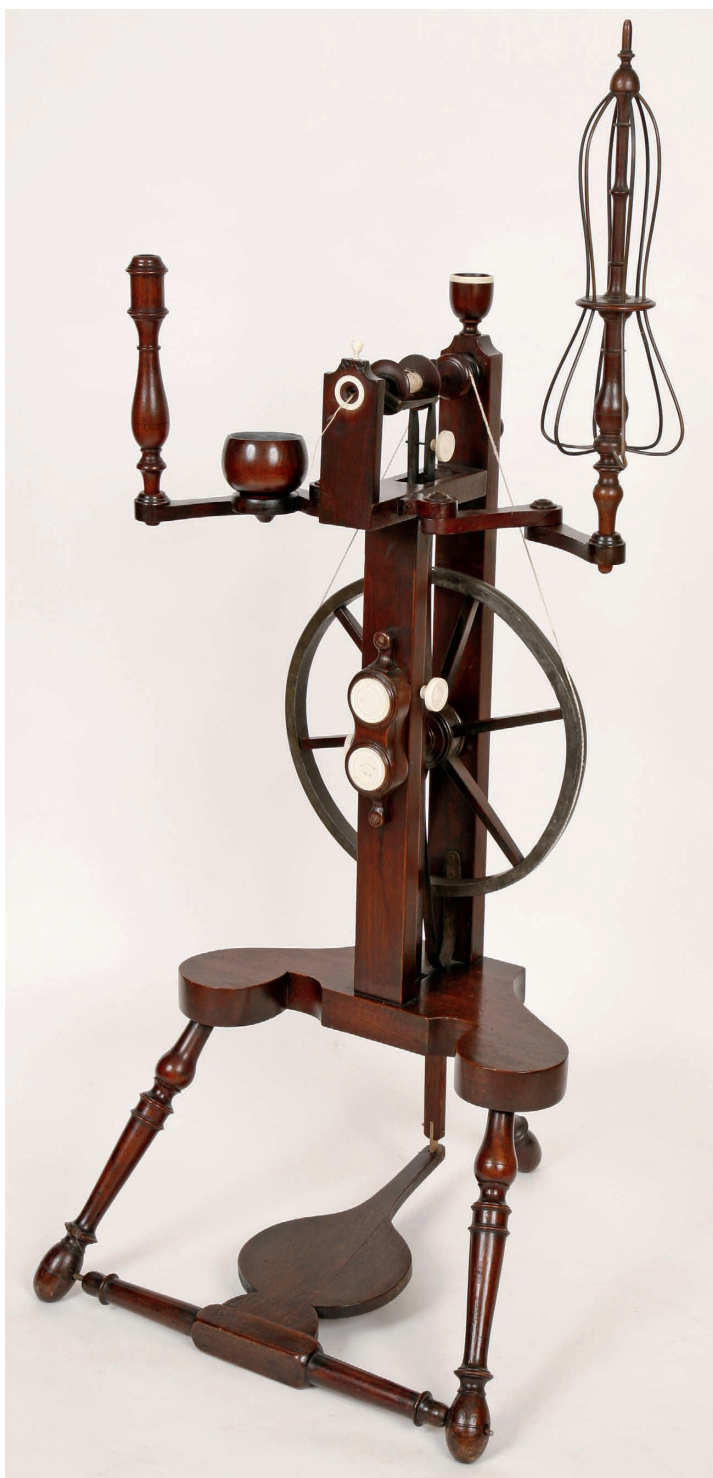
24 A Doughty spinning-wheel, probably c. 1800–13, possibly made by Marshall, Martha Doughty's partner, with the Antis Mark 3 mechanism. The authors
