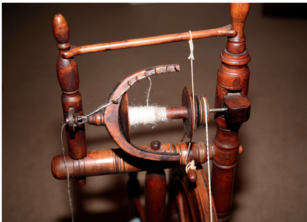
7 Traditional bobbin/flyer with ‘Scotch’ tension arrangement. The authors
