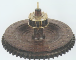
Striking train, second wheel, made from oak, lignum vitae and brass
