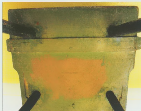
Fig. 4 The wany edge of the middle board
