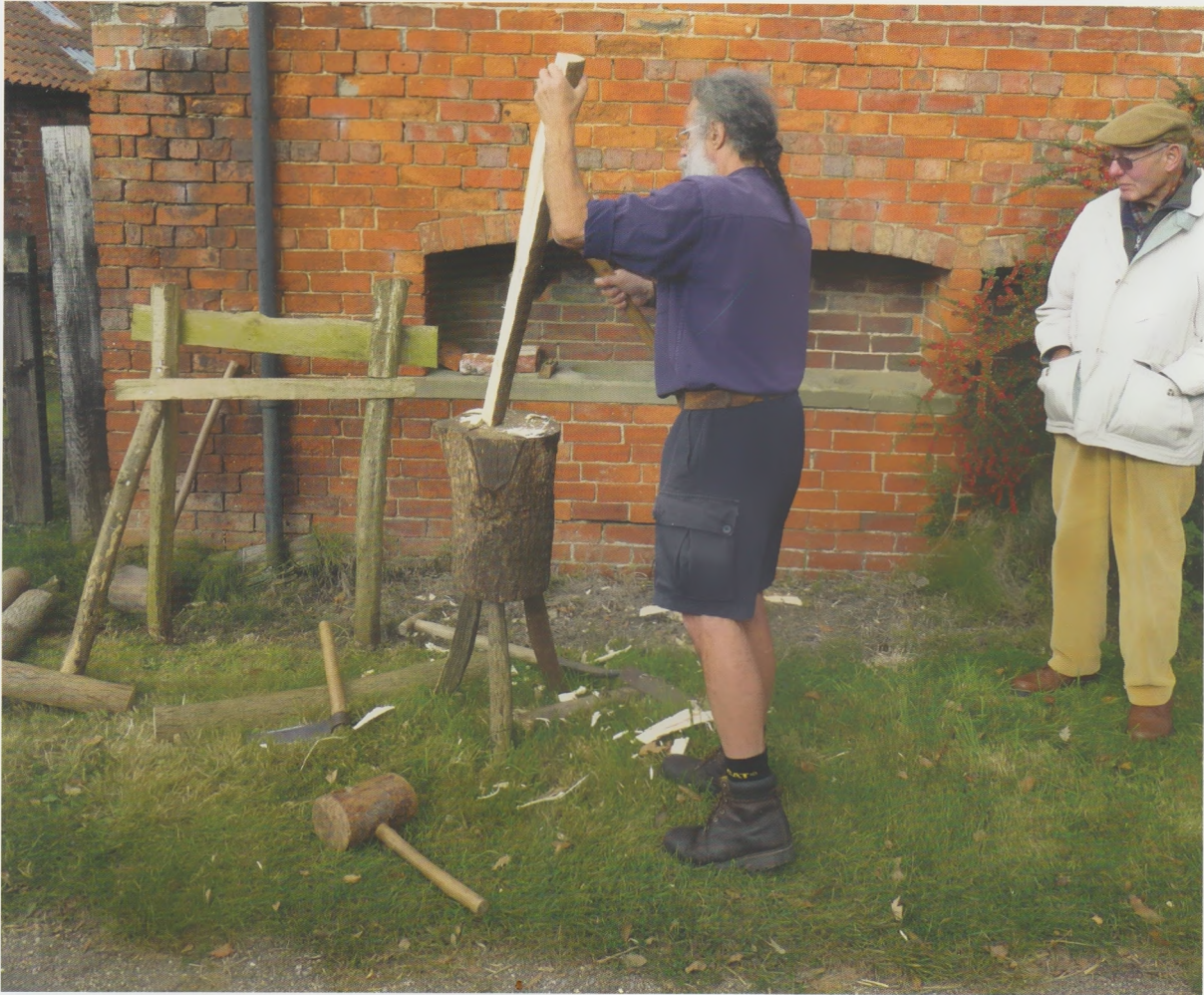
Fig. 1 Rob Ley demonstrating the technique of riving coppiced ash
