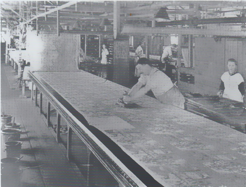
Fig. 5 Hand-block printing c. 1916. Note the young female 'tierer' on the right preparing the blocks for use
