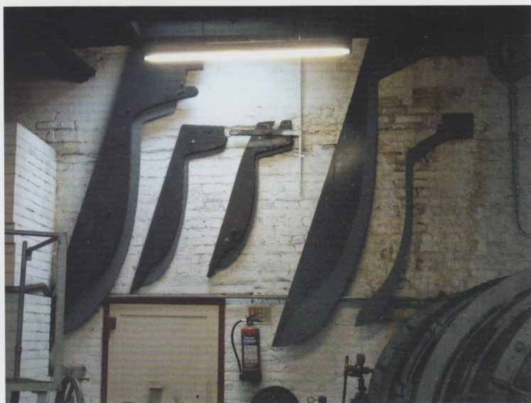
A range of profilers hanging on the wall; the largest is for Big Ben.
