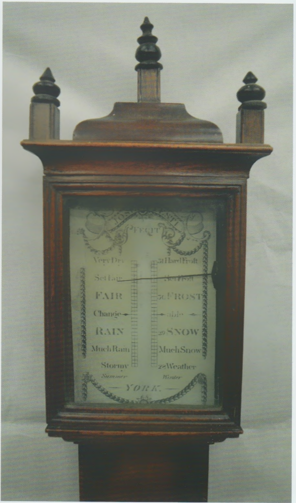
The barometer case after the removal of the mercury tube, showing the printed paper scale of Joseph Testi
