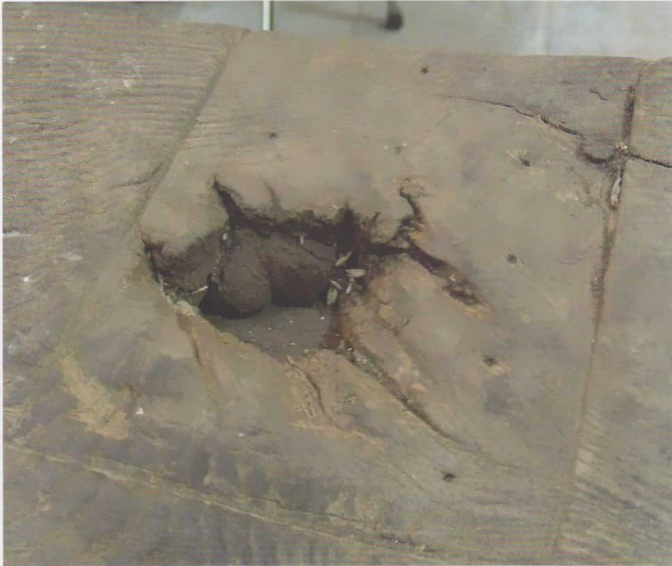
Nail holes show the position of a former patch on the table top
