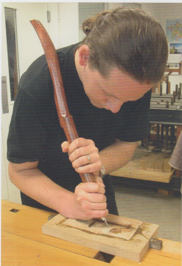
A craftsman using an inlay or shoulder knife to cut precisely shaped cavities in the solid wood
