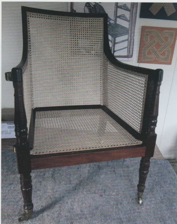
Re-caned chair showing the mahogany fillets at the junction of the back and arm panels with the seat panel
