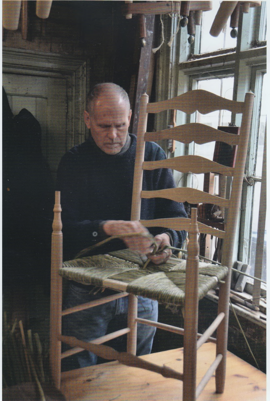
Lawrence Neal rushing a chair. Note that he is rushing the seat before putting on the arms as it makes the rushing easier. Photo Neil MacLennan
