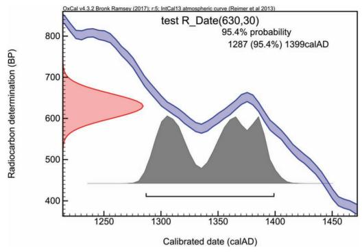
The red area represents the actual measured amount of radiocarbon in a sample, with its error spread. When extended across to the calibration curve (blue) at this particular position, several possible dates are derived, with the probability for any given calibrated date shown by the grey area.
