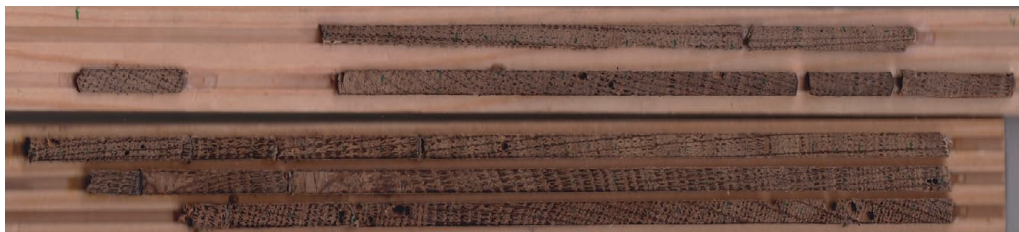
Figure 2 Scan of the cores (01–05 top to bottom) showing the worm holes and breaks encountered.
