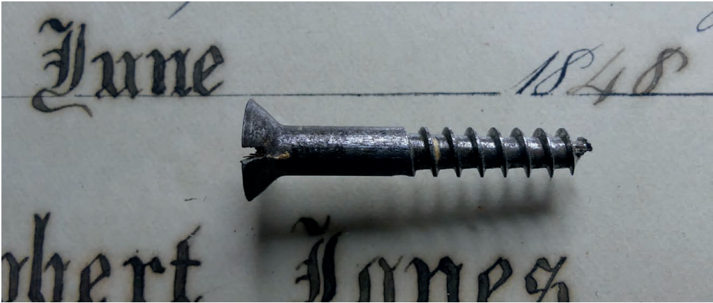
22 Transitional screw type found in a cabinet made in Adelaide for the Independent Order of Rechabites (Southern Star Tent No. 5), 1848. State Library of South Australia SRG 164/137/10
